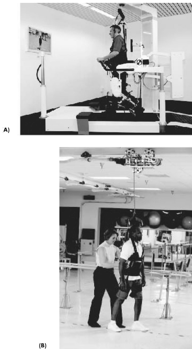
Figure 2. (A) Lokomat robotic exoskeleton (Hocoma AG, Volketswil, Switzerland) assists patients as they walk on a treadmill. (B) ZeroG overground gait and balance training system (Aretech, LLC, Ashburn, Virginia).
